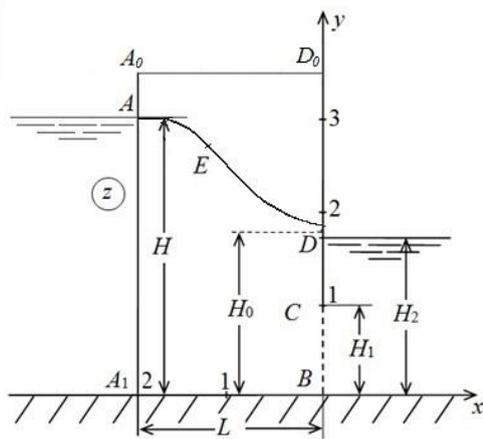
**Figure 1:** A picture of the current in a rectangular jumper with a screen, calculated at the  $\varepsilon = 0.5$ ,  $H = 3$ ,  $L = 2$ ,  $H_1 = 1$ ,  $H_2 = 1.4$ .
