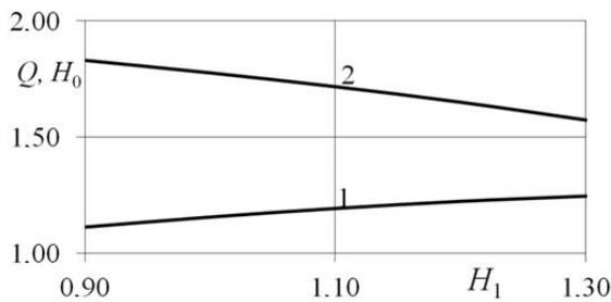
**Figure 3:** The flow of the jumper and the  $H_0$  exit point of the free  $H_0$  surface from the length of the  $H_1$  filter.
